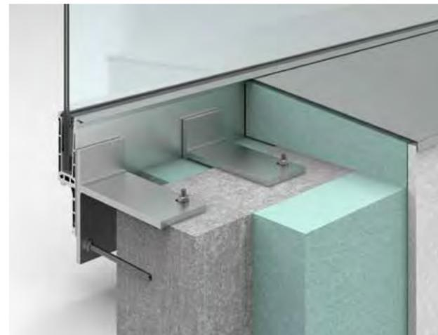
MONTAGE AN GEDÄMMTER ATTIKA
